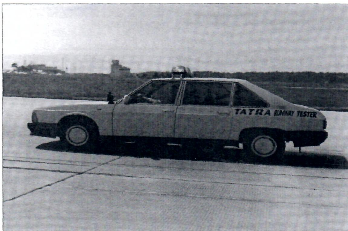
Figure 5-12. Tatra Friction Tester
